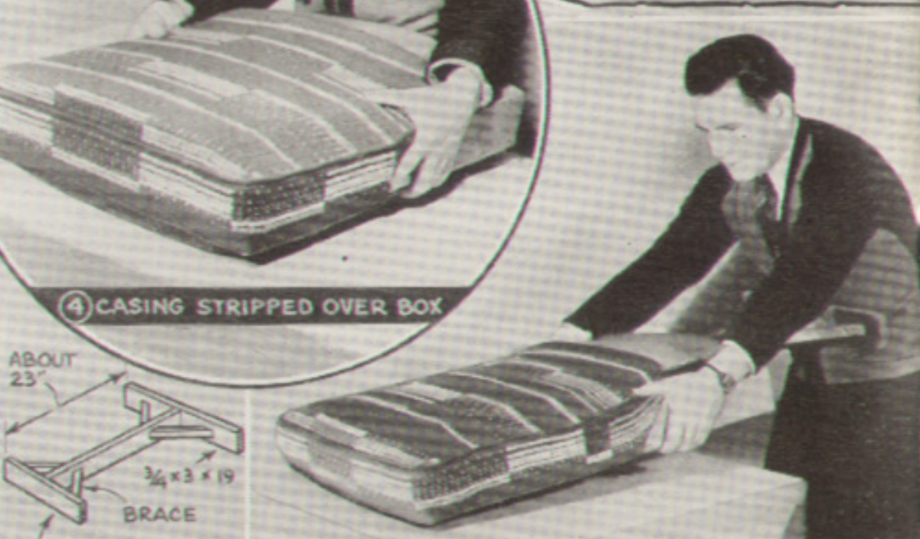
4 CASING STRIPPED OVER BOX 5 RAMROD HOLDS SPRING AS BOX IS REMOVED
