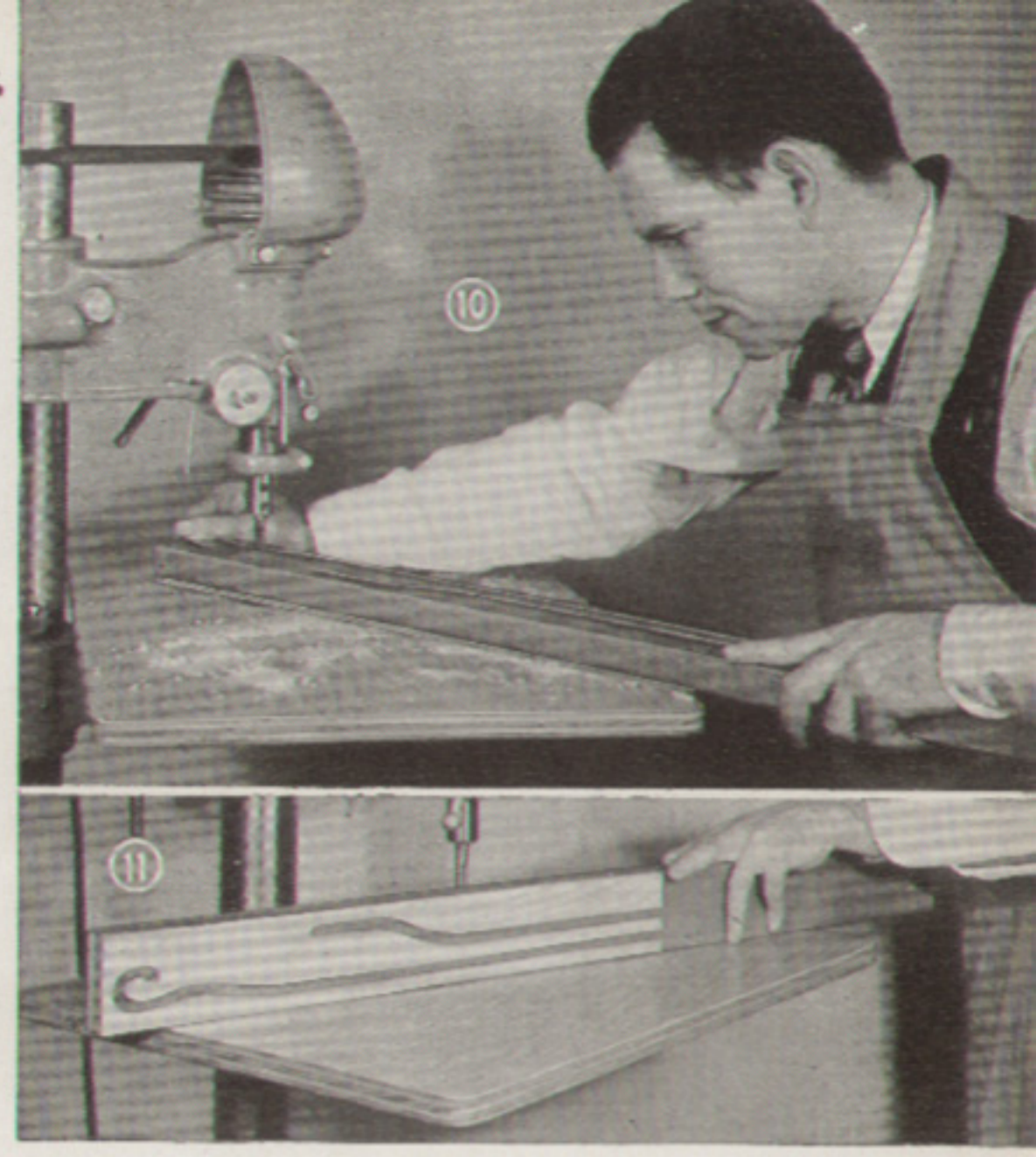
A pattern of the grooves in the bearer is made to permit routing on the drill press. Since the work is symmetrical, the pattern need be only a little over half full length.
