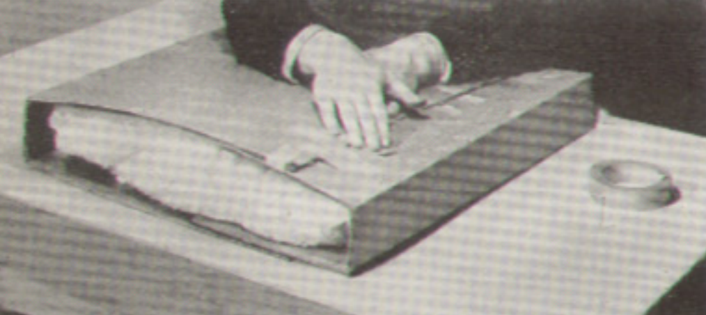
3 BOX CLOSED AND FASTENED WITH GUMMED TAPE
